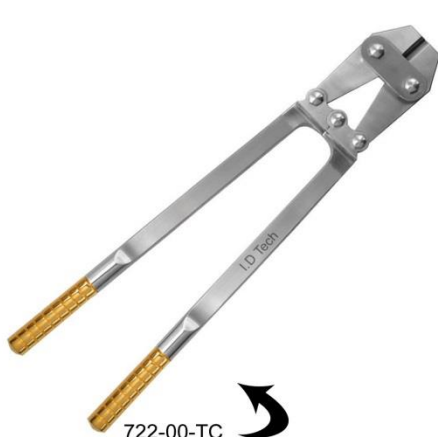
722-00-TC Heavy Duty Pin Cutting Plier TC Gold A: 30 cm / 12" Cut Upto 3mm B: 47 cm / 18 1/2" Cut Upto 5mm C: 56 cm / 22" Cut Upto 6mm D: 60 cm / 24" Cut Upto 7mm
